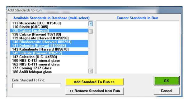
Click the **Add Standard to Run >>** button to move these standards into the current run. Standards may be added one at a time or the user may multi-select standards by holding down the <Ctrl> button on the keyboard as standards are selected. Double clicking each entry will also send the standard to the other column in the dialog window.
