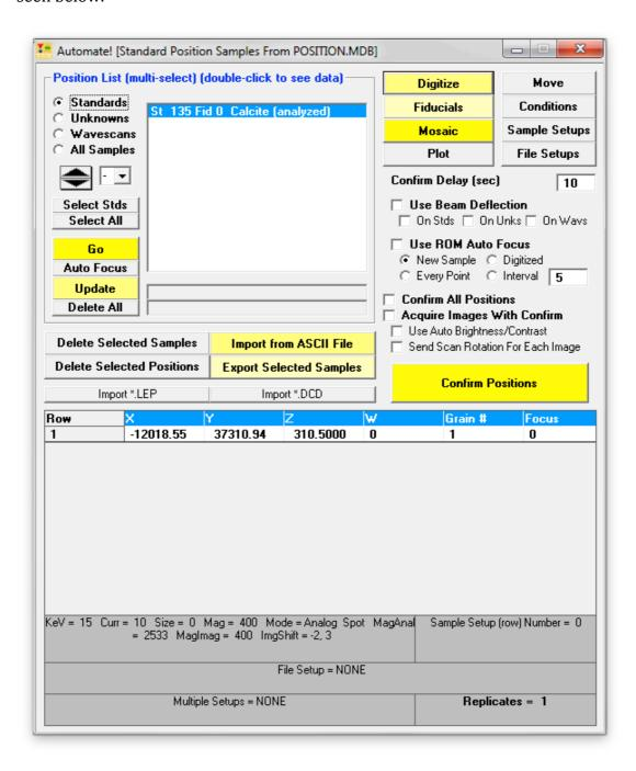
Note, that although only one position per standard needs to be digitized, if additional points are digitized, PROBE FOR EPMA will automatically utilize them. Otherwise, PROBE FOR EPMA will simply increment the stage X position for each additional acquisition required.
