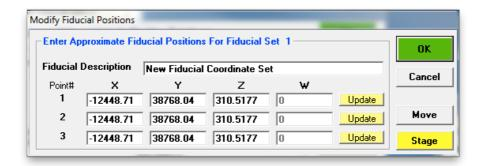
Type in a *Fiducial Description*. Enter the nominal coordinates or click on **Stage** to open the Stage Map! window to move to each of the three fiducial marks on the standard mount, determining their approximate coordinates and click the respective **Update** buttons. The following window will result.
