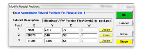
This action causes the stage motors to drive to the first fiducial coordinate.
