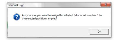
Again a message box is displayed indicating that subsequently digitized positions will have the new fiducial set assigned, for example in case further standard positions need to be added. This assignment can be changed at any stage later using the same procedure:
