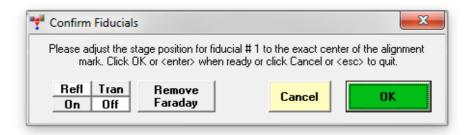
The computer will drive to each of the three fiducial marks for centering. Clicking the **OK** button after the third fiducial mark opens the **FiducialsVerifyFiducials** window. Click this **OK** button.
