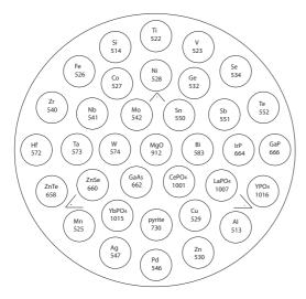
Other features like distinct grain edges in the corners of the mount can also be used as fiducial markers. All markers should provide distinct features on a micron scale to allow for high accuracy positioning and extend far enough in depth to be preserved after successive repolishing of the surface.
