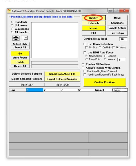
This opens the **Digitize Sample Positions** dialog box. The *Standard Compositions Added to Run* list box contains the standards already added to the run.
