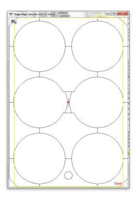
The distance between these positions is around 27 mm both in X and Y direction. The exact amount of shift depends on several parameters like exact diameter of the standard mount, order in which the two Allen screws holding the mount are fixed, etc.
