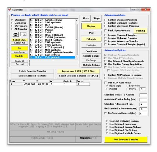
Repeat the same loading procedure for the other standard position files required for use in the automation. After clicking the **Import from ASCII File** button, the **AutomateImportFile** window opens.
