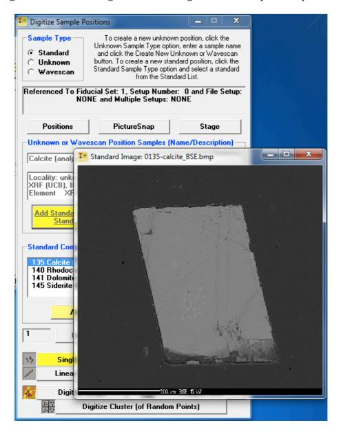
To digitize a random point on this standard, click the **Single Point(s)** button of the **Digitize Sample Positions** dialog box to record the current XYZ coordinates for this grain. The coordinates of this standard in the **Automate!** dialog box are seen below.
