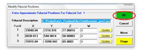
As before, adjust and confirm the stage positions for each of the 3 fiducials:
