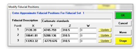
Click the **OK** button when done. This creates a new entry in the **Select Fiducial Set** list box as shown below. Select (highlight) the new fiducial set and click the **Confirm** button to initiate a precise centering of the three fiducial marks.
