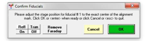
After completion, the software will again display the message box with information about the sample tilt and then a box confirming the update of the positions based on the new fiducial coordinates:
