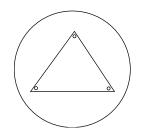
The fiducial marks should be deep enough to withstand repeated re-polishing but small enough to be precise for relocation of the digitized coordinates.
