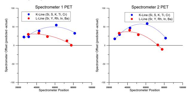
Spectrometer Calibration Offsets for Ka and La lines on PET Crystals
