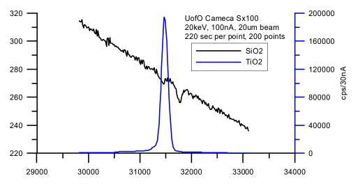
For example, spectrometer analyzing crystals have secondary lattice reflection planes which will produce small artifacts ("holes") in the spectrum, some directly underneath the analytical peak (depending on the mounting orientation). This produces a systematic accuracy error in trace element analyses that can easily exceed the precision of the measurement even with moderate beam current and count times.
