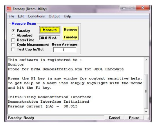
The Faraday application is a small utility useful for controlling the faraday cup and making beam current measurements. It has a cycle control which can be used to continuously monitor the beam current for stability measurements.
