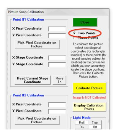
6. In Point #1 Calibration section, click Pick Pixel Coordinate on Picture:
