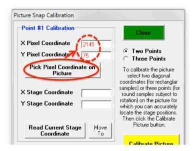
9. Drive stage to the actual position of this feature, for example using joystick, trackball or similar. Click *Read Current Stage Coordinate*:
