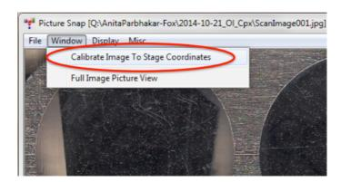
5. The **Picture Snap Calibration** Window opens. All pixel and stage coordinate fields should be empty. To use 2 reference points for calibration, ensure the radio button for **Two Points** is selected:
