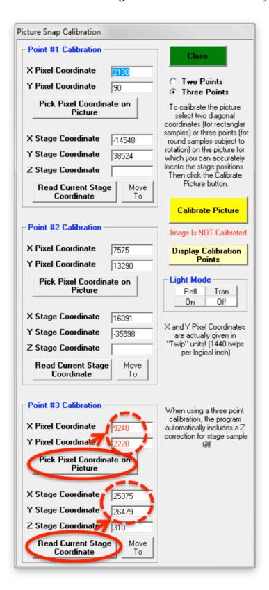
19. Click *Calibrate Picture* again and click *OK* in the message box to save the new 3-point calibration. The "Image Is Calibrated" message in the **Picture Snap Calibration** window indicates that the new calibration can now be used for navigation:
