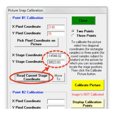
10. Repeat steps 6 to 9 for *Point #2* in the respective section, using a feature in the bottom right area of the image, for example a sharp corner of a grain:
