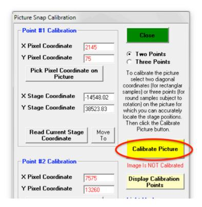
13. The calibration will be saved into a separate small ASCII text file with .ACQ extension. As long as the .ACQ file is kept together with the image file, PictureSnap will reload the calibration when the image is reopened. Click **OK**:
