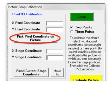
7. Now click onto the feature to be used as first reference point in the picture. Note: This feature should be close to one corner of the imported image and be easily recognisable in both the imported image as well as the live imaging of the instrument (SE/BSE or built-in light microscope).
