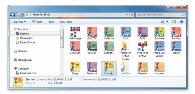
Alternatively, select **Startwin** in the Probe Software group of the Windows Start Menu, or locate and double click on STARTWIN in the Probe for EPMA application directory, which is usually C:\Probe Software\Probe for EPMA under Windows Vista and Windows 7, or C:\Program Files\Probe Software\Probe for EPMA for older operating systems.
