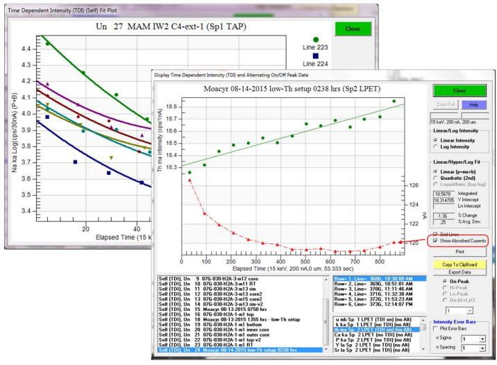
Easily correct for sensitive samples by automatic acquisition and correction for intensity changes over time by correcting for both intensity loss or gain.
